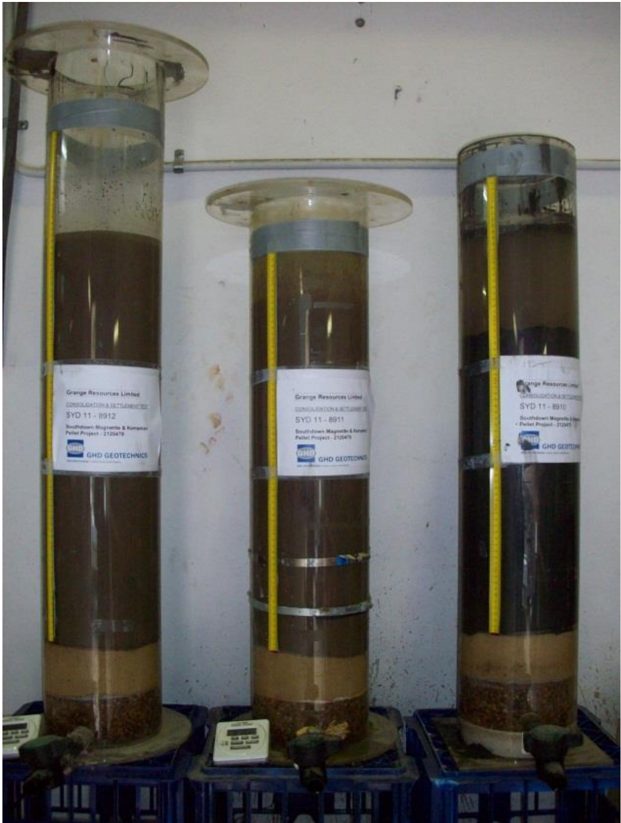
Figure 1 Column settlement and consolidation test.
