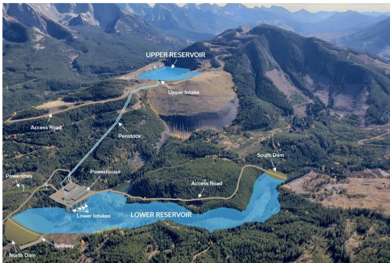
Figure 2 Overlay rendering of the PHES configuration at Tent Mountain (courtesy of Montem)
