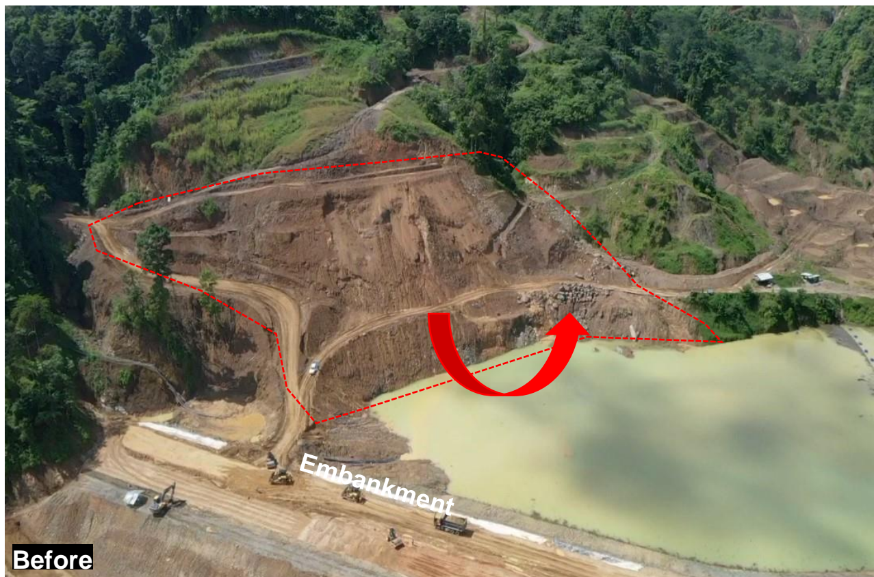
Figure 2 Upstream batter noted to be potentially unstable
