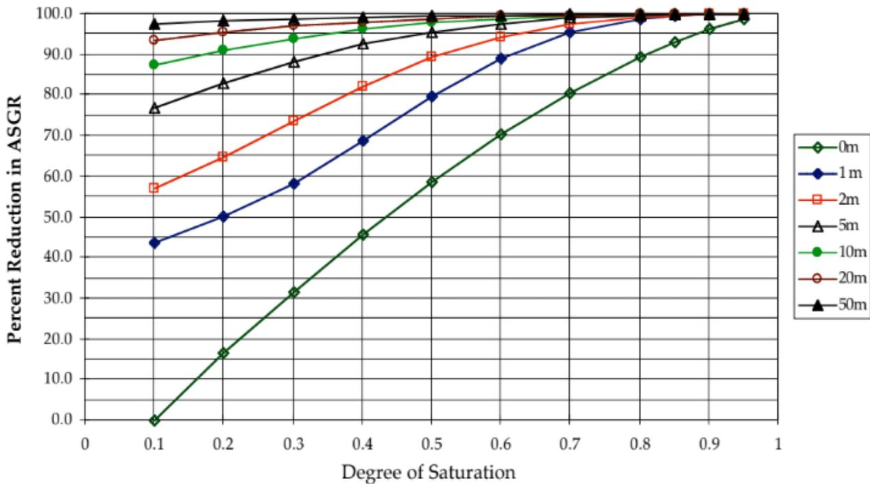
Figure 3 Cover saturation versus reduction in ASGR (Miller, 1998).
