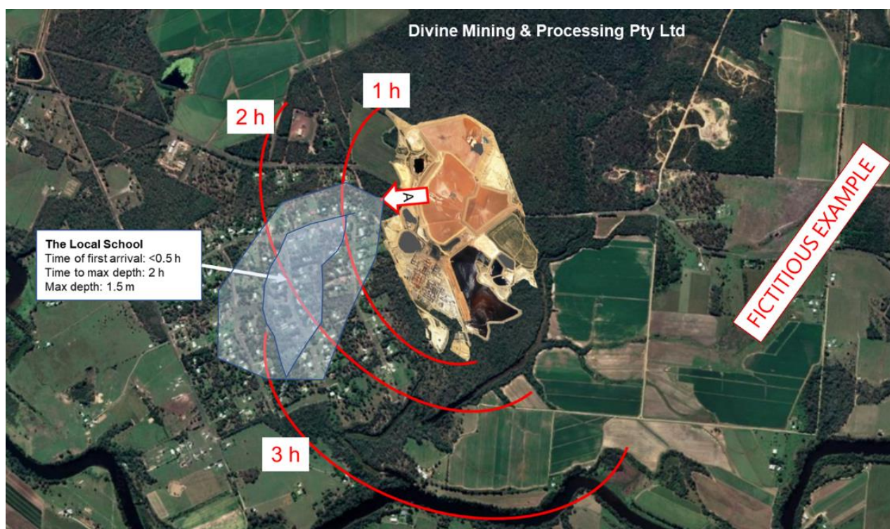
Figure 4 Individual inundation map with points of interest and isochrones, showing estimated time of arrival. Fictitious example
